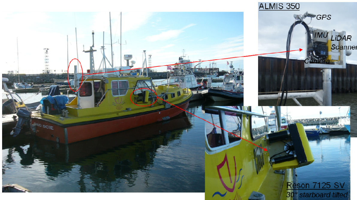
Figure 2: Integrated MBES / lidar system mounted on the CIDCO's survey vessel.
